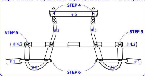
**Step 3**: Connect the U (#2) & L (#3) bars together, then connect them to bar # 4 but leave the outer 2 holes open. Do not tighten up any nuts / screws yet, just leave them loosely connected.
