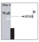
Place wall anchors into holes.
