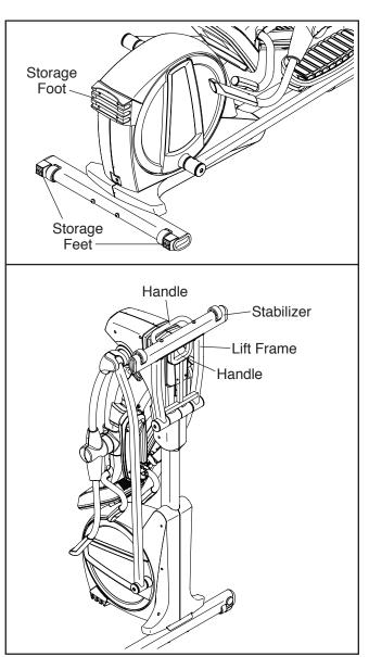
To lower the elliptical for use, first hold the handle on the lift frame with one hand and hold the front stabilizer with your other hand. Next, pull the frame towards you and lower it until you can reach the handle on the front stabilizer. Then, hold the handle on the front stabilizer with both hands and finish lowering the elliptical to the floor.
