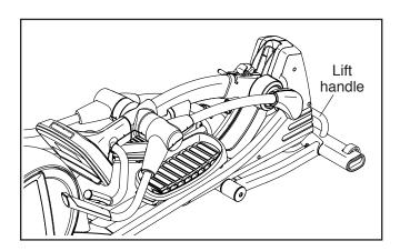
When you are finished moving the elliptical, lift the upright to the vertical position and tighten the upright knob.
