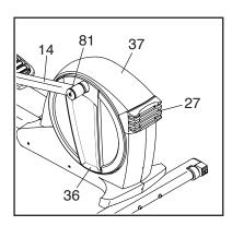
Remove the four M4 x 16mm Screws (not shown) from the Large Storage Foot (27), and then remove the Large Storage Foot. Remove the two M4 x 16mm Screws (not shown) from the Top Shield (37), and then use a standard screwdriver to pry the Top Shield upward off the elliptical. Then, pry the left Pedal Disc (36) off the elliptical.
