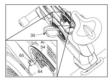
Next, rotate the Left Crank Arm (35) until a Magnet (54) is aligned with the Reed Switch (64). Slide the Reed Switch slightly toward or away from the Magnet. Then, retighten the M4 x 19mm Screw (65).
