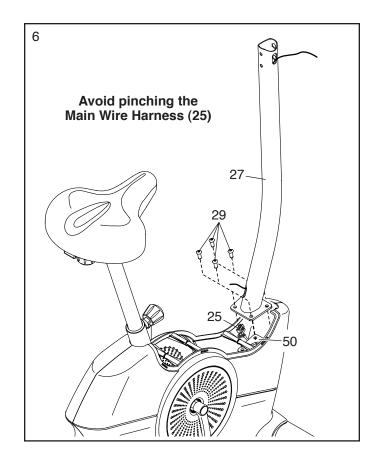
Locate the lower end of the wire tie in the Upright (27). Tie the wire tie to the Main Wire Harness (25). Then, pull the upper end of the wire tie until the Main Wire Harness is routed through the Upright and out of the indicated hole.
