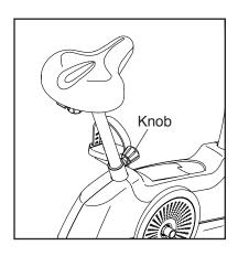
post knob. Move the seat post upward or downward slightly to make sure that the seat post knob is engaged in one of the adjustment holes.
