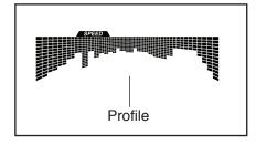
The flashing segment of the profile represents the current segment of the workout. The height of the flashing segment indicates the target speed or the incline level for the current segment.
