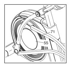
Next, turn the left Crank Arm (20) until one of the Magnets (43) on the Pulley (19) is aligned with the Reed Switch (38). Then, loosen, but do not remove, the two M4 x 16mm Screws (104), slide the Reed Switch (38) slightly closer to or away from the Magnet (43), and retighten the Screws.
