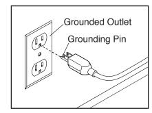
A temporary adapter may be used to connect the power cord to a 2-pole receptacle as shown at the right if a properly grounded outlet is not available.
