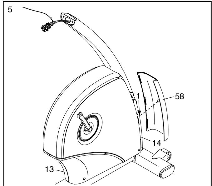
6. Orient the Upright Cover (57) as shown. Hold the Upright Cover near the Upright (2), and insert the wires upward through the Upright Cover.
