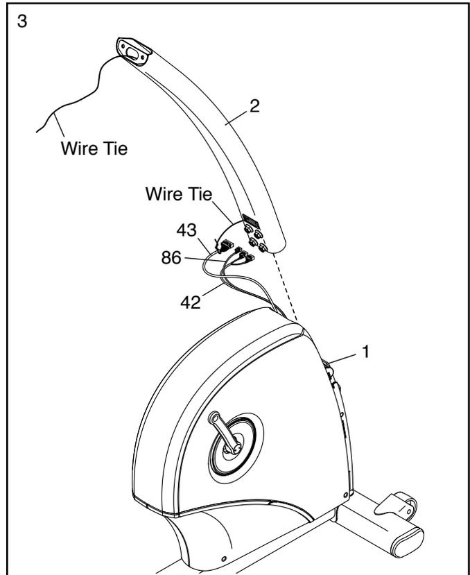
4. **Tip: Avoid pinching the wires.** Slide the Upright (2) onto the Frame (1).
