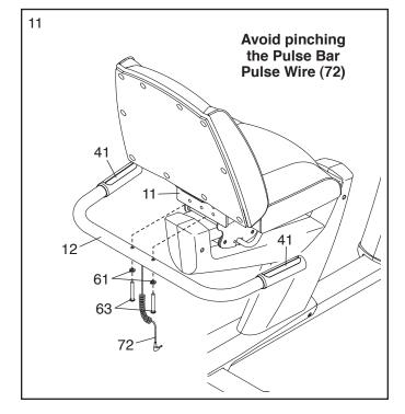
12. Plug the Pulse Bar Pulse Wire (72) into the Frame Pulse Receptacle (75) located in the Left Seat Shield (24).
