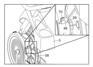
Locate the Reed Switch (46). Turn the Pulley (58) until a Magnet (29) is aligned with the Reed Switch. Next, loosen, but do not remove, the indicated M4 x 13mm Flange Screw (70). Slide the Reed Switch slightly closer to or away from the Magnet, and then retighten the Screw. Plug in the power adapter and turn the Pulley for a moment.
