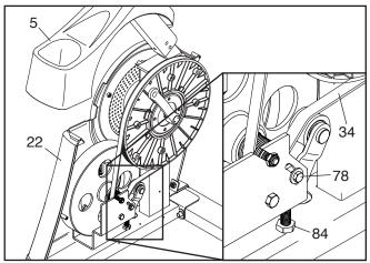
Then, remove all the screws from the Left and Right Front Shields (22, not shown); there are three sizes of screws in the Front Shields—note which size of screw you remove from each hole. Then, gently pull the Right Front Shield away from the frame.
