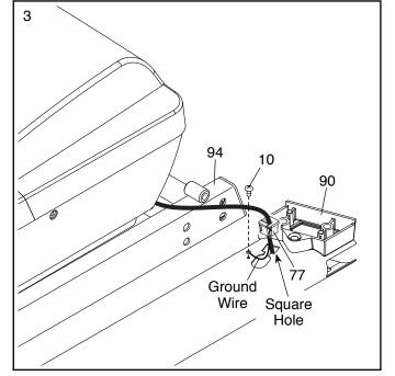
4. Hold the Right Upright (90) against the Base (94). Be careful not to pinch the wires. Partially tighten three 3/8" x 4" Screws (7) with three 3/8" Star Washers (13) into the Right Upright and the Base; do not fully tighten the Screws yet.
