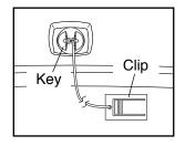
IMPORTANT: In an emergency, the key can be pulled from the console, causing the walking belt to slow to a stop. Test the clip by carefully taking a few steps backward; if the key is not pulled from the console, adjust the position of the clip.
