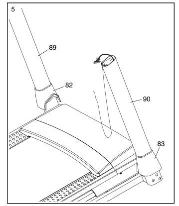
Identify the left handrail assembly (A). Attach the left handrail assembly to the Left Upright (89) with two 5/16" x 2 1/2" Screws (28) and two 5/16" Star Washers (11); do not fully tighten the Screws yet.
