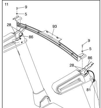
12. With the help of a second person, hold the console assembly near the Handrails (86) (only one side is shown).
