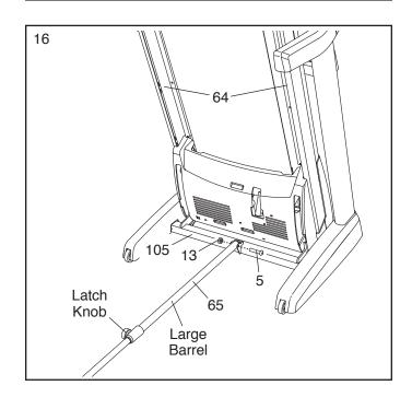
17. Attach the upper end of the Storage Latch (65) to the Frame (64) with a 3/8" x 1 3/4" Bolt (7) and a 3/8" Nut (13). Note: It may be necessary to move the Frame back and forth to align the Storage Latch with the Base (not shown).
