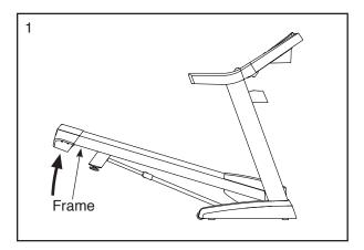
2. Raise the frame until the latch knob locks in the storage position. **CAUTION:** Make sure that the latch knob locks.
