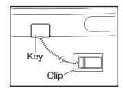
the displays will light. IMPORTANT: In an emergency, the key can be pulled from the console, causing the walking belt to slow to a stop. Test the clip by carefully taking a few steps backward; if the key is not pulled from the console, adjust the position of the clip.
