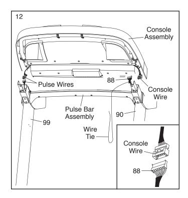
13. Insert the pulse wires and the Upright Wire (not shown) into the Handrails (92, 93) as you set the console assembly on the Handrails.
