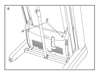
Lower the treadmill (see HOW TO LOWER THE TREADMILL FOR USE on page 29). Remove the three #8 x 3/4" Screws (2). Carefully pivot the Motor Hood (72) off.
