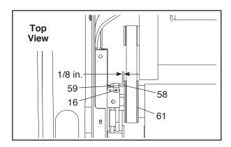
SYMPTOM: The incline of the treadmill does not change correctly
